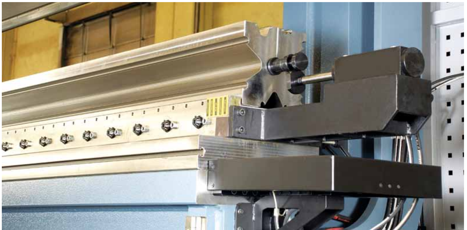
Hydraulic Bottom Tool Separation System
