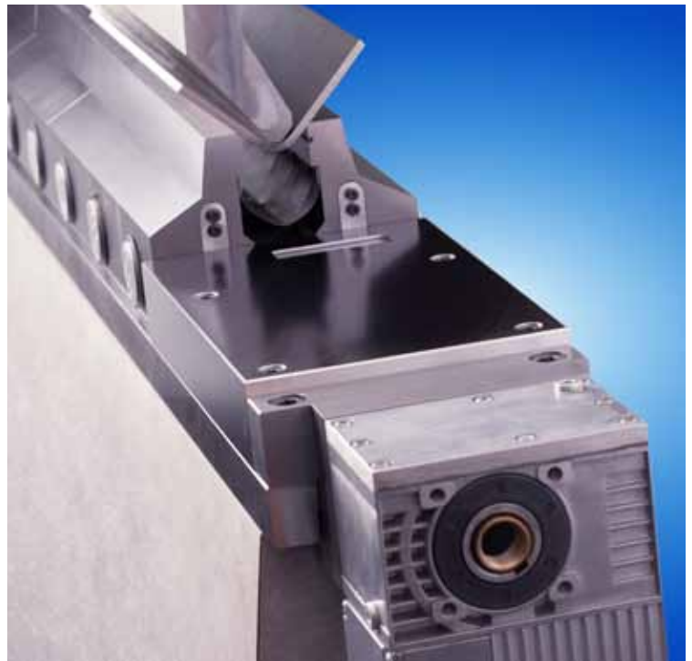
Bottom Tool CNC Adjustable System (Multi-V)
